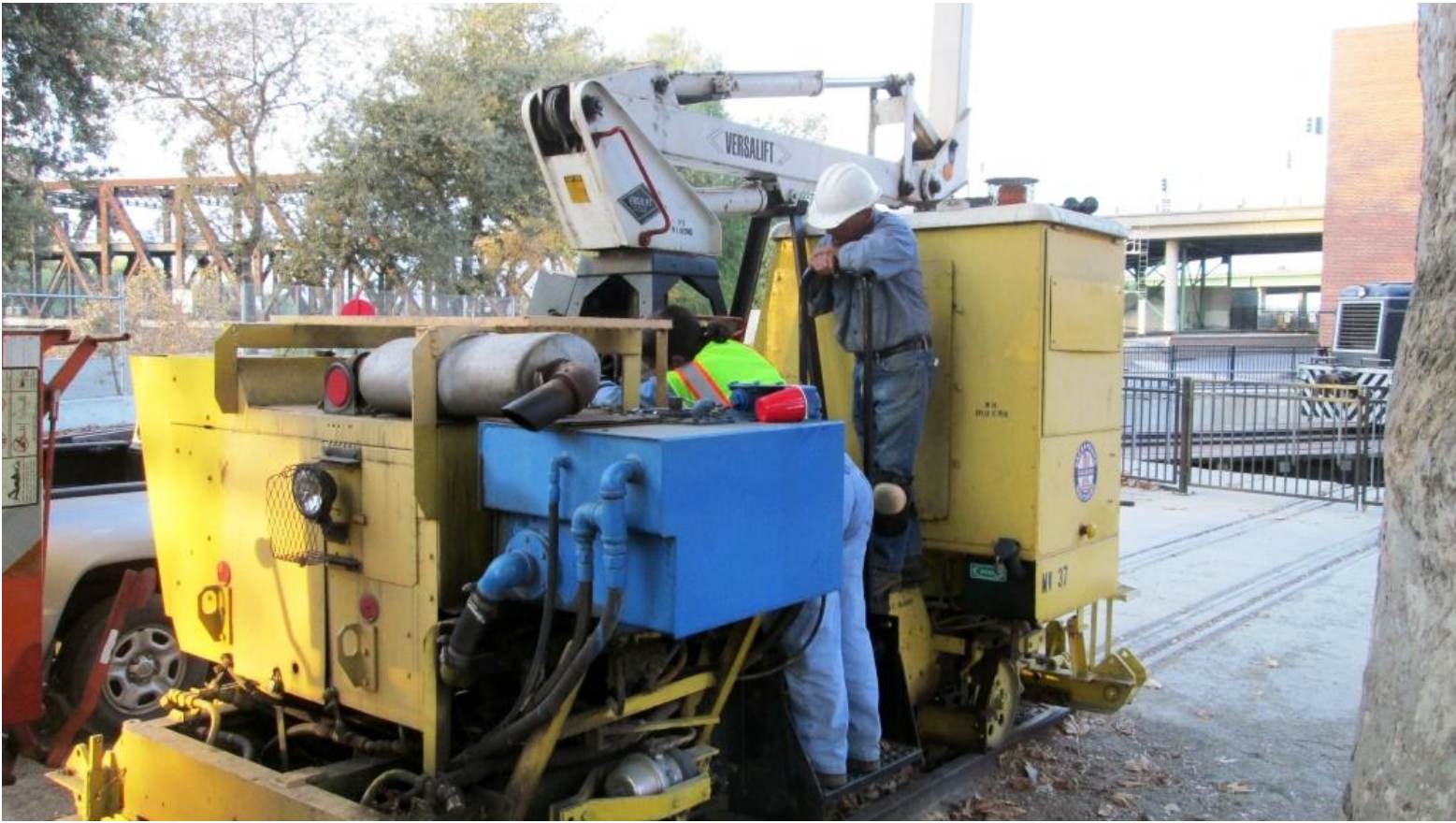
Heather and Mike replace the "spider" gear on the man-lift
