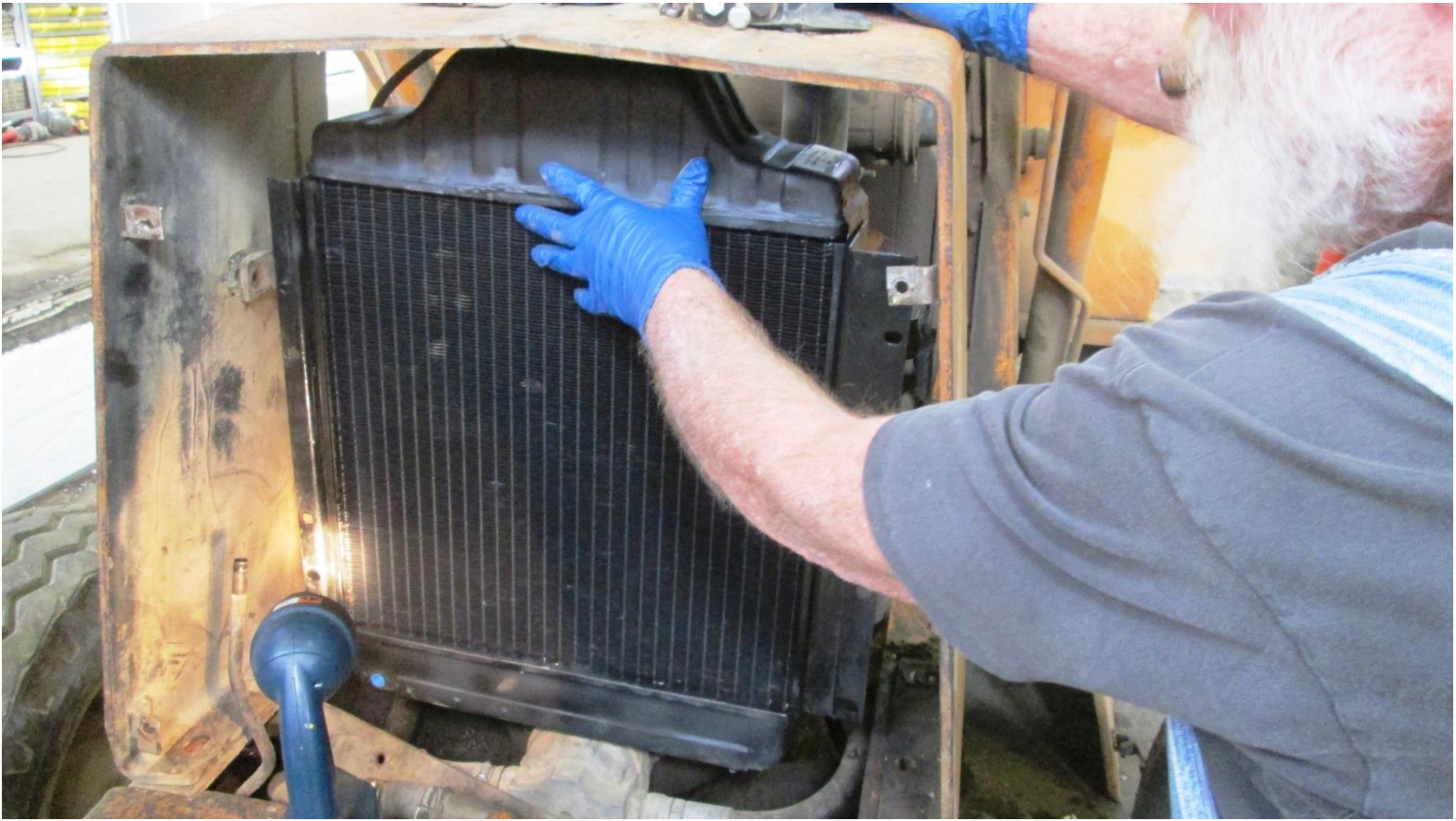
Pat prepares to remove the back-hoe's old radiator
