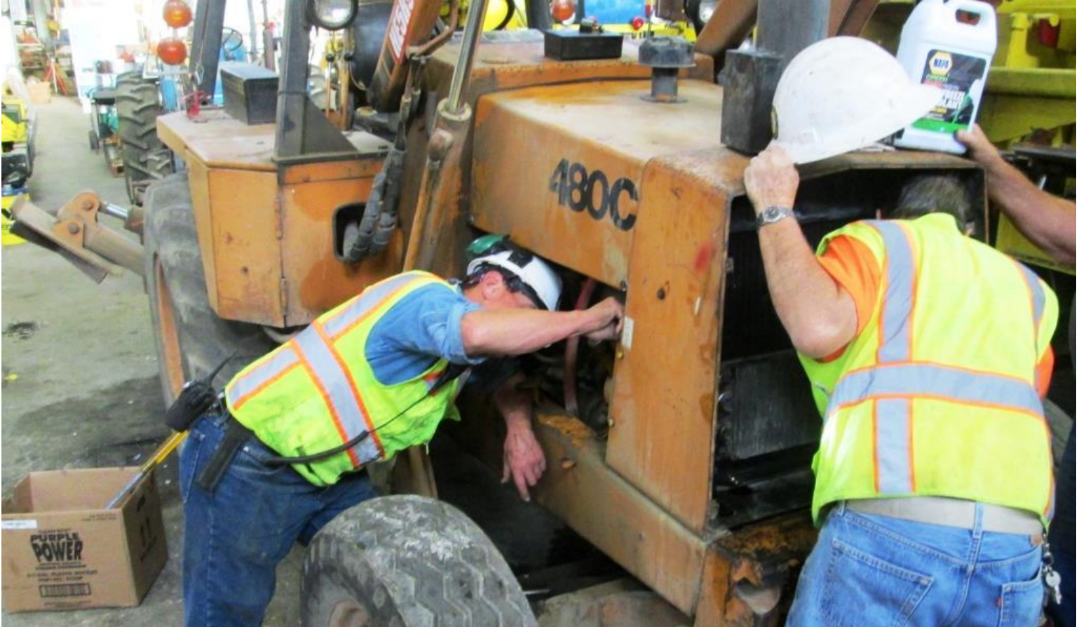
Joe and Mike H. get the install the new radiator in the back-hoe
